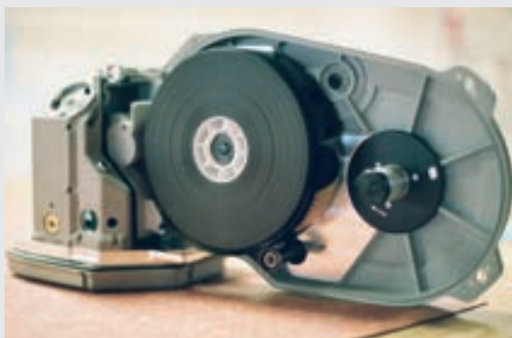
The first prototype of the Penelope 35 mm, open-hearted. At first, Jean-Pierre Beauviala dreamed of the possibility of adapting digital or film magazine - Photo Valentina Miraglia.
