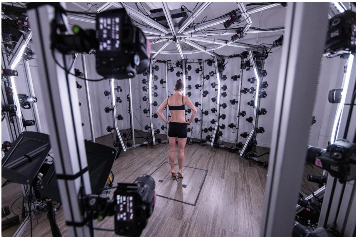
**Fig. 32.** 3D-scan photogrammetry studio.
