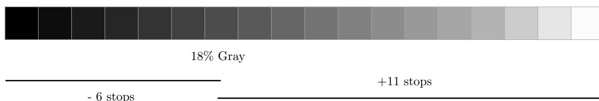
Figure 14 - Exposure range and stop repartition for film
