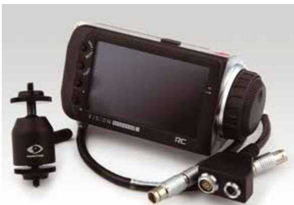
RCU-Miro Kit, Includes Phantom RCU, Mounting Bracket and Cables
